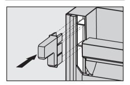
Fit the wall spacers onto the back of the appliance on the top left and right.
